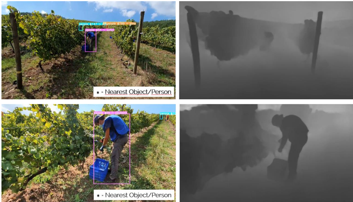
Figure 23. Output frames from PDLT app: RGB with detection info (left), monocular depth estimation (right)
