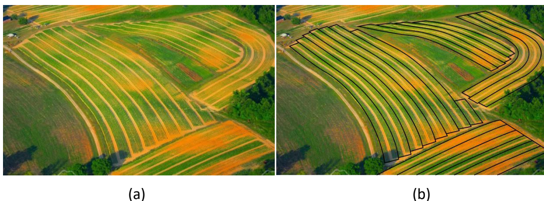
Figure 51 (a) Irregularly shaped fields with varying crop directions and (b) their representation on tracks
