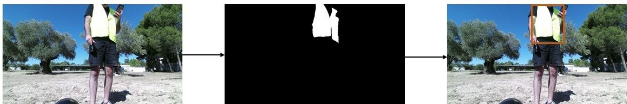
Figure 41. Operator detection system (RGB-D images)
