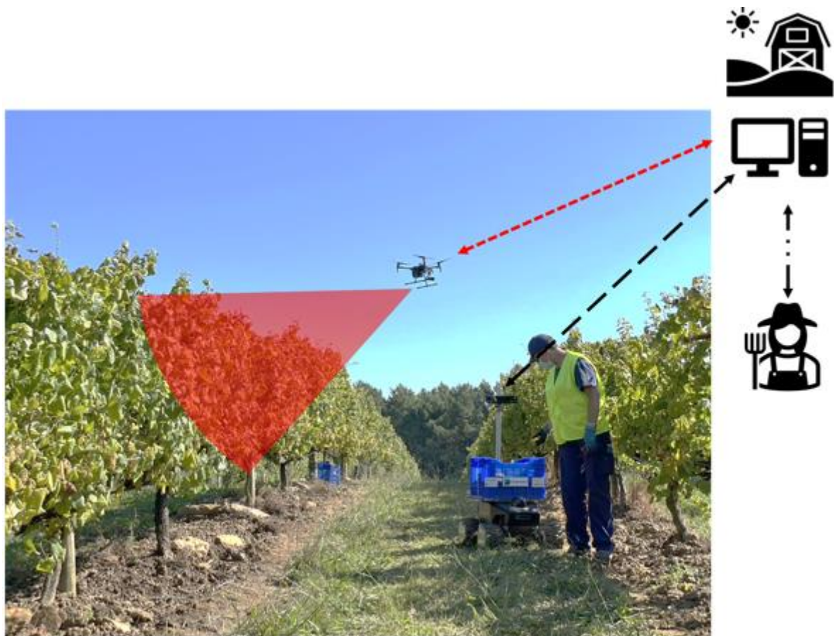
Figure 37. Representation of the process that ranges from data acquisition (from both UAV and UGV), to the detection of Botrytis and the consequent communication to the farmer
