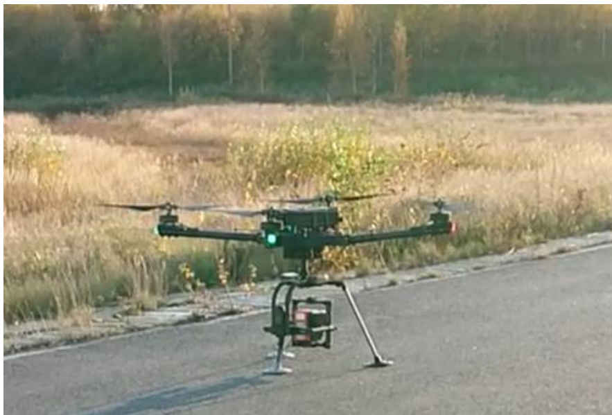
Figure 31. Backup drone: FreeFly AltaX drone with Specim AFX17 hyperspectral camera
