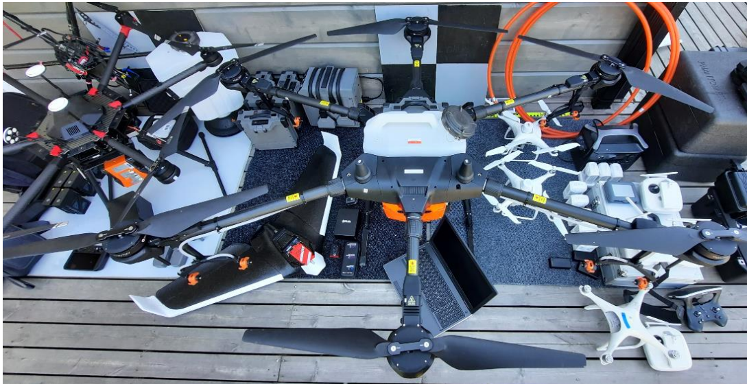
Figure 30. Luke's' drones for project purposes. From the left: DJI Matrice 600 pro and Specim AFX10 & AFX17, Parrot Disco Fixed wing, DJI Agras T-16 spraying drone, three different DJI Phantom 4 drones
