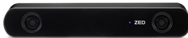
Figure 37. Zed2 stereo camera is used to detect the obstacles in front of the tractor (image source: https://www.stereolabs.com/zed-2/ )
