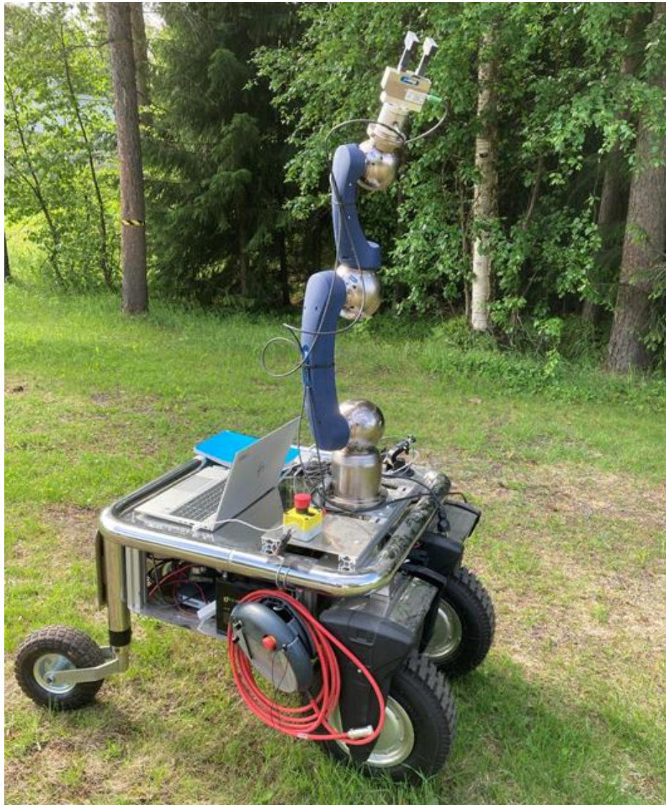
Figure 29. Test platform for weeding including a mobile robot platform (made by Probot Oy) with Schunk LWA 4 PB with force/torque sensor (ME MessSysteme GmbH) and compliant motion control
