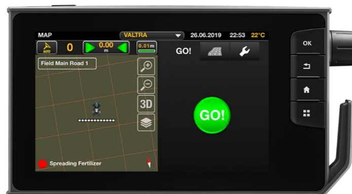
Figure 36. Valtra Guide commercial auto steering system. The same terminal is used to control other tractor functionalities and ISOBUS VT/TC. (image source: https://valtrateam.valtra.com/tekniikka/automaattiohjaus-uudistui/ )
