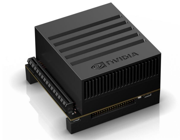
Figure 38. The machine vision software is run on NVIDIA Jetson AGX Xavier (image source: https://developer.nvidia.com/embedded/jetson-agx-xavier-developer-kit )
